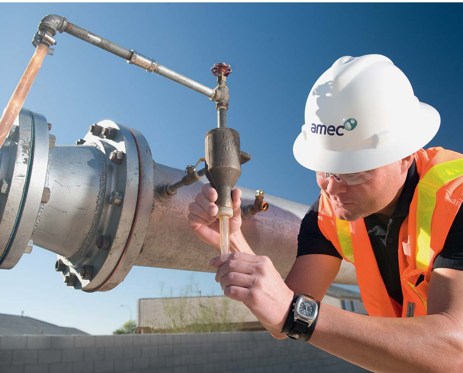
Chris Courtney, Senior Hydrogeologist, formerly with Geomatrix, collects a sand content measurement from a sand tester during pump testing
