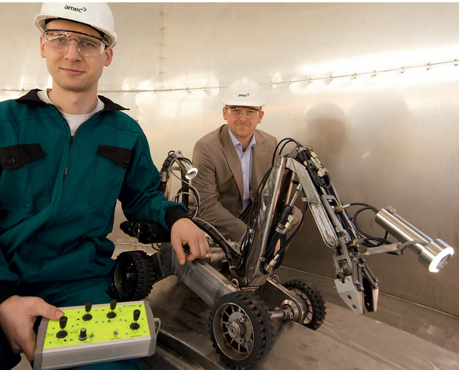
Left to right: Peter Mraz, Designer/ROV Operator and Pavol Stuller, Commercial and Business Development Manager, both formerly with AllDeco, with a remotely operated vehicle used in the removal of highly contaminated waste
